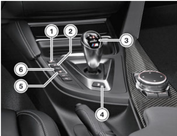
F82 GTS, M DCT Drivelogic gear selector switch and driving dynamics button (example BMW M4 Coupé)
